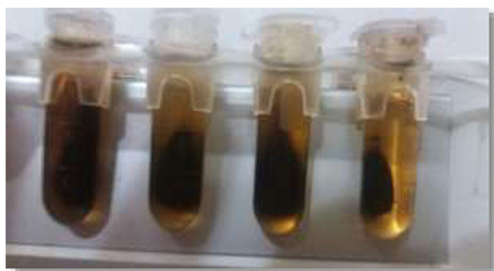
Fig. 1 The image of synthesized \text{Fe}_3\text{O}_4/\text{poly}(\text{SEMA-co-MMA}) nanocomposite in deionized water
