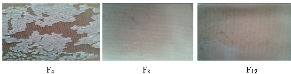
Fig. 2 Pictures of the films prepared by compression molding between hot plates at 230 °C and at a pressure of 1.5 MPa for 5 min of the samples obtained using 3.2 % of peroxide in the three series; i.e. F 4 , F 8 and F 12
