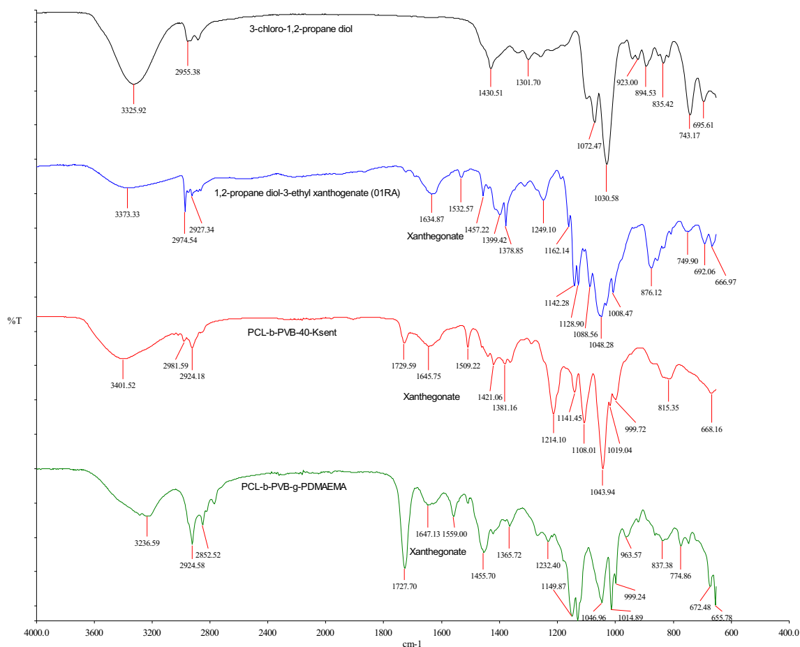
Fig. 5 The FT-IR spectra of 3-chloro 1,2-propane diol, 1, 2-propane diol-3-ethyl xanthogenate (01RA), PCL- b -PVB-40-Ksent, and PCL- b -PVB- g -PDMAEMA samples
