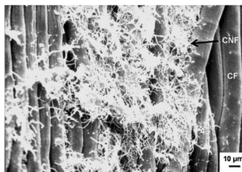
Fig. 5 Fracture surface of multi-scale composites showing distribution of CNFs
