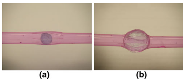
Fig. 43 Swelling of a spherical hydrogel inside a straw (with some local cuts). a Half-way wetted; b fully wetted. Reproduced with permission from VSP, an imprint of Brill [172]
