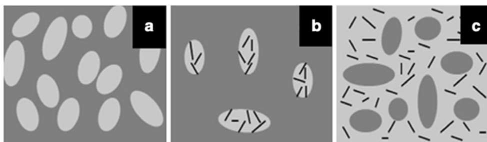
Fig. 2 Schematic representation of morphological state of blend-based nanocomposites: a polymer blend, b blend nanocomposite in which nanoparticles are localized in dispersed phase and c blend nanocomposite in which nanoparticles are localized in matrix phase
