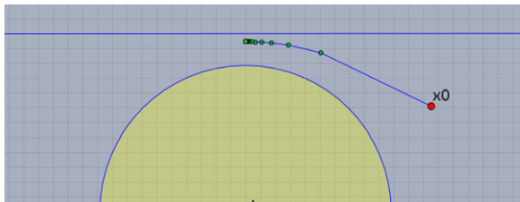
Fig. 4 An interactive Cinderella applet showing the cyclic Douglas–Rachford method applied to the case of a non-intersecting ball and a line. The method appears convergent to a point whose projections onto the constraint sets form a best approximation pair. Each green dot represents a cyclic Douglas–Rachford iteration (Color figure online)
