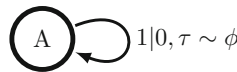
Fig. 2 The smallest generative model of a continuous-time renewal process consists of a single causal state. The transition is labeled p|s, \tau \sim \Pr(T) , denoting the transition is taken with probability p , emits symbol s for duration \tau distributed according to \Pr(T) . The length T_i = \tau of periods of silence (corresponding to output symbol 0) are drawn independently, identically distributed (IID) from probability density \phi(t)
