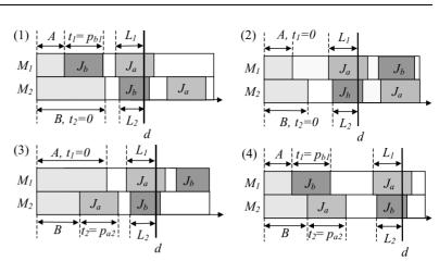
$M_2$ . Moreover, there are exactly  $t_1$ ,  $t_2$  units of early tasks and exactly  $L_1$ ,  $L_2$  units of partially late tasks on machines  $M_1$ and  $M_2$ , respectively. As already mentioned, there are three possible cases, when set  $J^P$  contains two, one, or none job. Taking into account the fact that all parameters of function  $f_{\bar{n}+1}(A, t_1, L_1, B, t_2, L_2)$  are bounded by O(d), the calculation of the initial conditions for any set  $J^P$  takes  $O(d^6)$  time.
