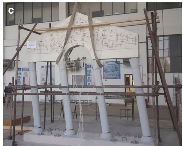
18); b oriented collapse of columns (computational model, after Hinzen 2009/2010), Fig 14); (c): set of columns just before oriented collapse (experimental, after Nikolić et al 2019).
