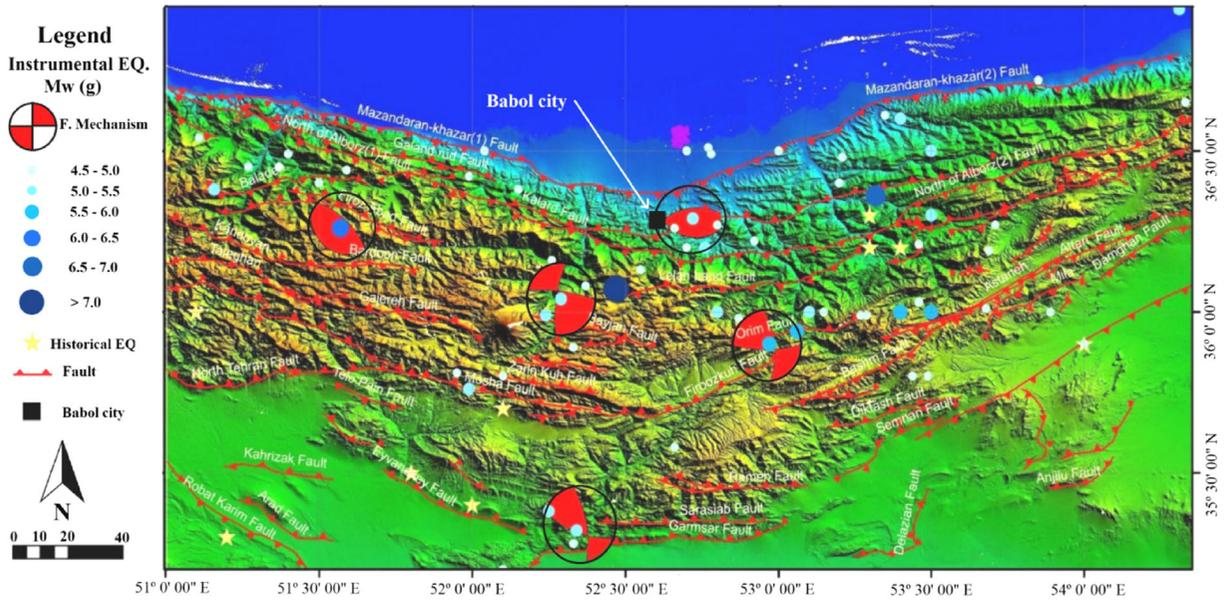
**Fig. 1** Location and magnitude of earthquakes, faults, and their mechanism near Babol City
