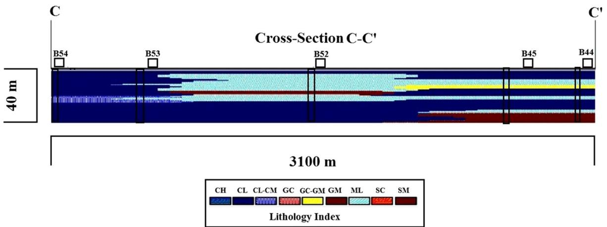
**Fig. 9** Cross section C-C'
