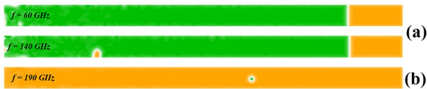
Fig. 2 a Formation of domain walls at frequencies f = 60 \text{ GHz} , 140 \text{ GHz} ; b the location of the skyrmion (velocity is slowed down) at f = 190 \text{ GHz} . All the snapshots have been taken at time t = 40 \text{ ns}
