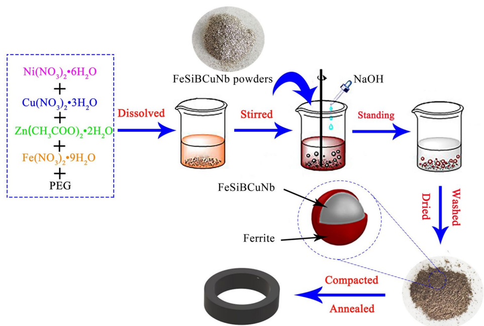
Fig. 1 Schematic illustration of \text{NiCuZnFe}_2\text{O}_4 coating prepared by chemical coprecipitation
