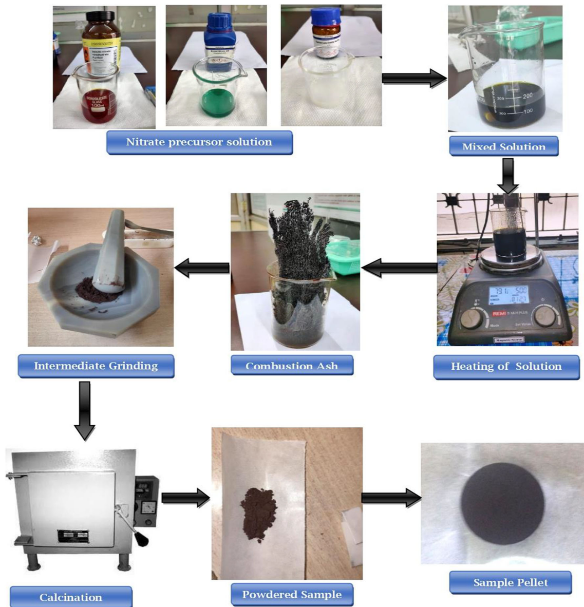
Fig. 1 Flow chart of synthesis of \text{NiFe}_{2-x}\text{Sm}_x\text{O}_4 ceramics using self-propagating sol-gel autocombustion method
