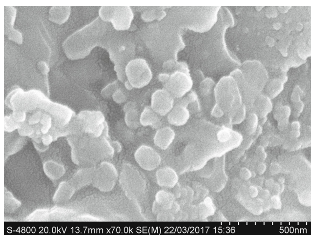
(a) FE-SEM images of cobalt ferrite nanoparticles.
