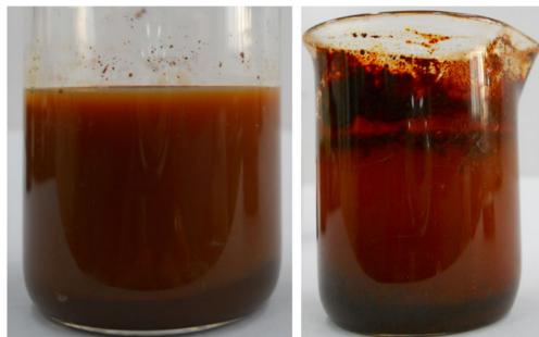
Fig. 26 Phenomenon of hydrocarbon-based ferrofluid stirred by NaOH at pH = 14
