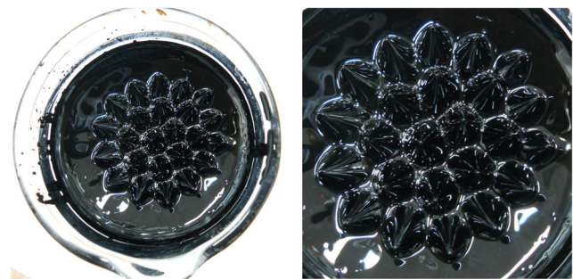
Fig. 2 Peak pattern of perfluoropolyether oil-based ferrofluid in applied magnetic field
