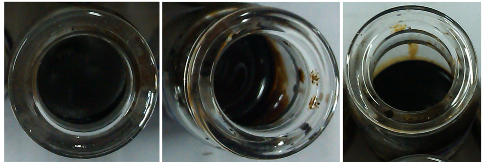
Fig. 5 Apparent state of water based ferrofluid, ester-based ferrofluid and perfluoropolyether oil-based ferrofluid at -40 °C
