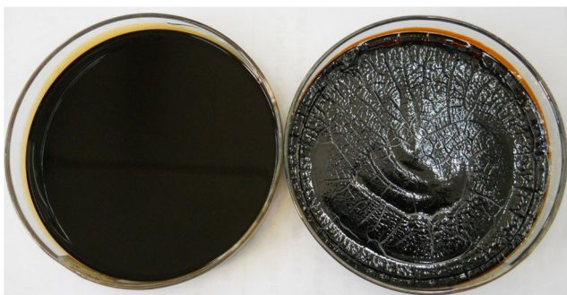
Fig. 4 Phenomena of perfluoropolyether oil-based ferrofluid and water-based ferrofluids after volatilization at 80 °C in atmospheric pressure
