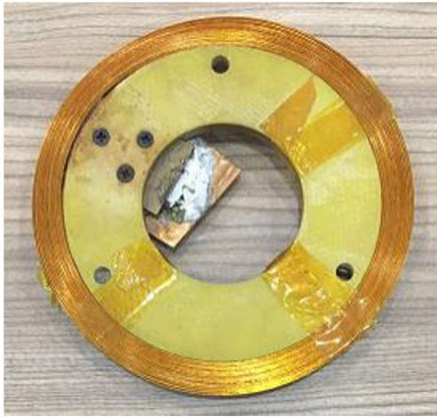
Fig. 3 Photograph of the experimental single pancake coil
