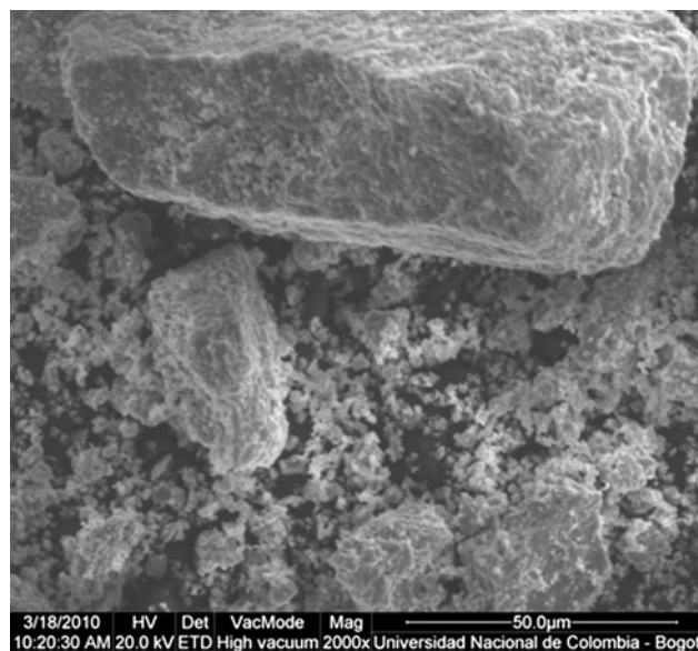
Fig. 2 SEM micrograph of \text{La}_2\text{SrCo}_2\text{FeO}_9 obtained from ETD detector (secondary electrons)
