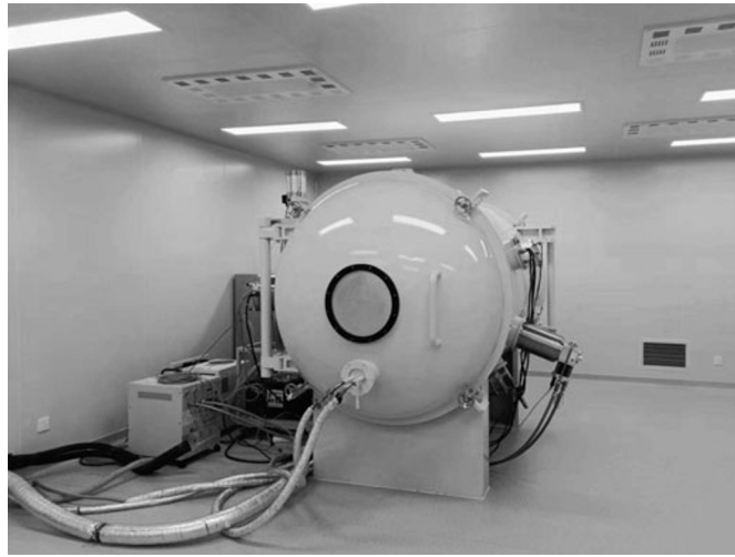
Fig. 4. Test of equivalent black-body temperature of the system. Vacuum chamber equipment.
