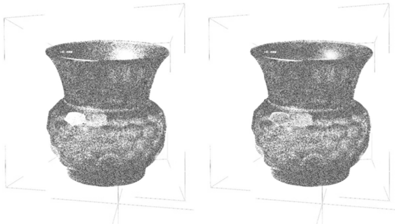
Fig. 4. Comparison of point cloud integrity generated by two methods: laser scanning (on the left) and proposed algorithm (on the right).
