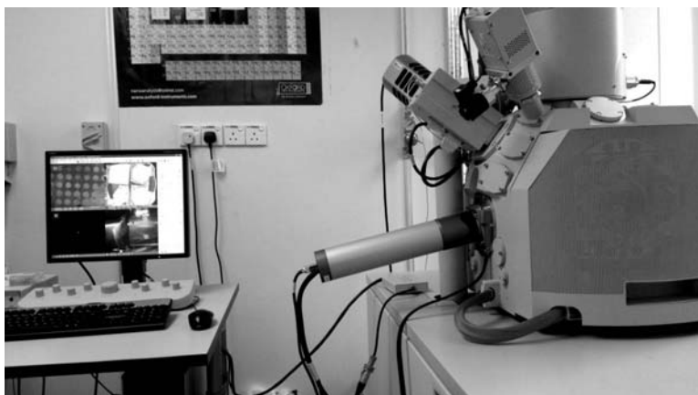
Fig. 3. Nova NanoSEM 450 with integrated EDX system to perform elemental composition analysis on the targeted region of interest. Here, computer unit used for image morphology and EDX analysis (a) and NanoSEM 450 chamber (b).
