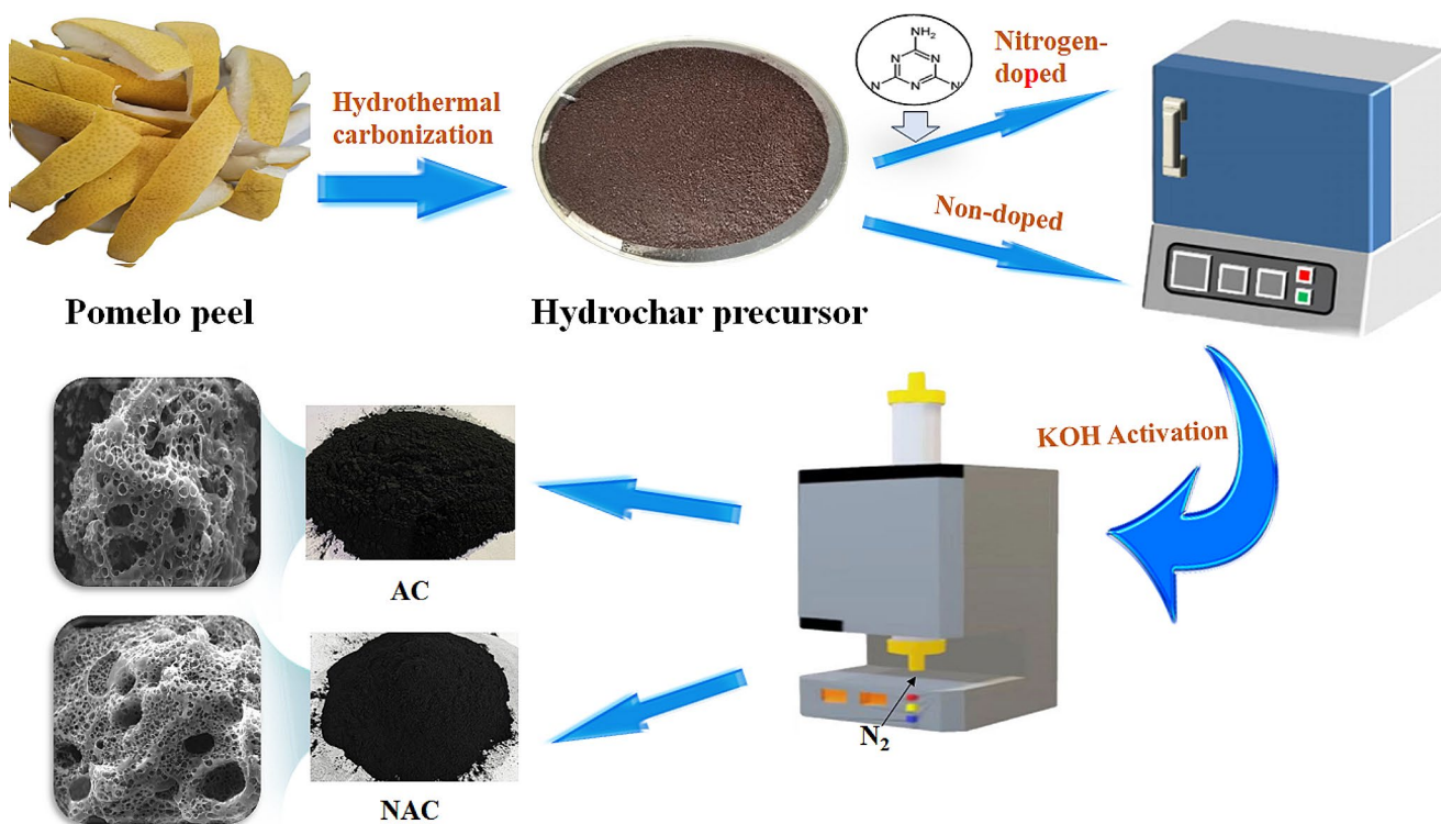
Fig. 1 Schematic illustration of the preparation of NAC and AC
