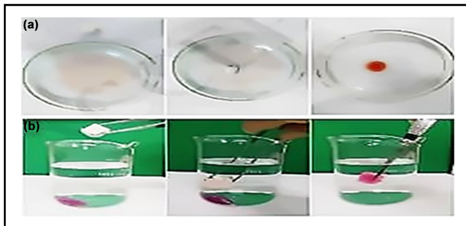
Fig. 10 A Schematic of absorption process of synthesized aerogel A oily substances, B and organic solvent [85]
