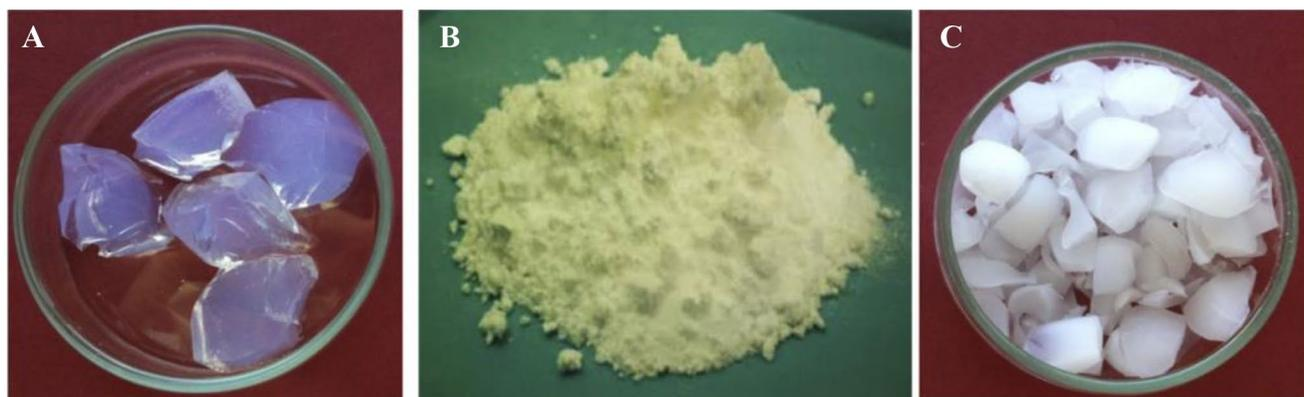
**Fig. 2** Photographs of the laboratory-synthesized silica aerogels: **a** inorganic aerogel produced in monolithic form; **b** hybrid aerogel produced in powder; **c** hybrid aerogel produced in monolithic form. Reprinted with permission from Ref. [6]. Copyright Elsevier B.V. 2019
