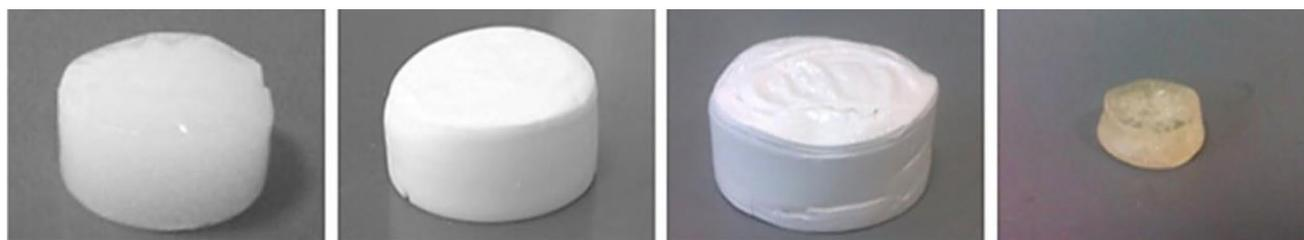
**Fig. 4** The effect of drying on a hydrogel obtained from cellulose solution. From left to right; hydrogel, aerogel (supercritical drying), cryogel (freeze drying) and xerogel (vacuum drying). Reproduced with permission from Ref. [28]. Springer International Publishing AG
