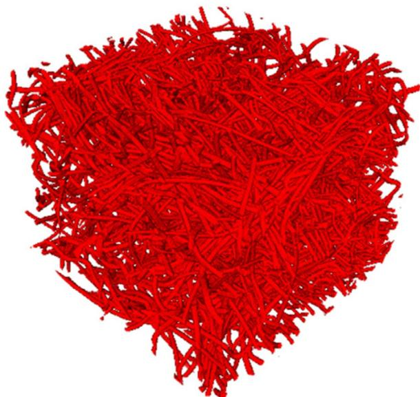
**Fig. 11** The untreated nonwoven fabrics geometry. Reproduced with permission from Ref. [103] Copyright 2019
