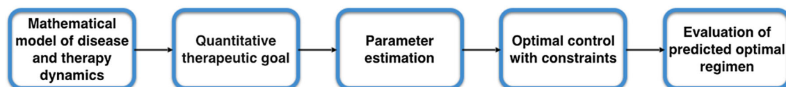
Fig. 1 Steps in optimization of drug regimens. Evaluation can be performed by running preclinical (animal) or clinical (human) studies and comparing outcomes to the optimal control predictions.
