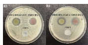
Fig. 6 Photos of antibacterial activity of the fabricated bio-based films in the disc diffusion method against (a) S.aureus , (b) E.coli
