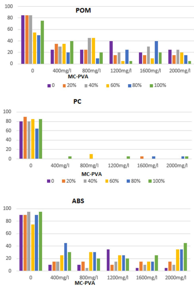
Fig. 4 The poly oxy methylene (POM), polycarbonate (PC) and acrylonitrile butadiene styrene (ABS) flotation (%) at different concentrations of MC-PVA for various microwave power levels (%). The flotation tank media pH was kept as 6.5 at ambient temperature. All plastics were irradiated by microwaves for 20 s before introducing to flotation tank
