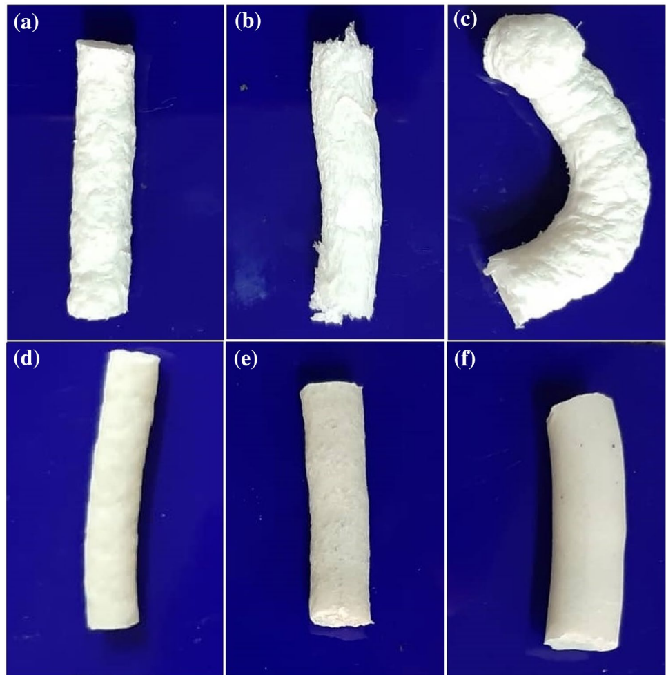
Fig. 7 TPS/PS blend foam with the optimized formulation of TPS. a F0, b F20, c F40, d F60, e F80 and f F100
