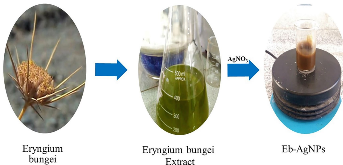
Fig. 1 Synthesis of silver nanoparticles (Ag-NPs) by Eryngium bungei Boiss extract
