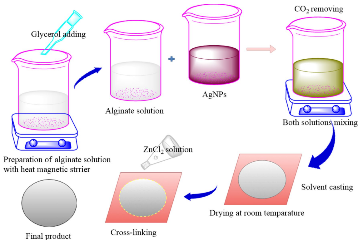
Fig. 2 A schematic diagram of sodium alginate and AgNPs incorporated films preparation
