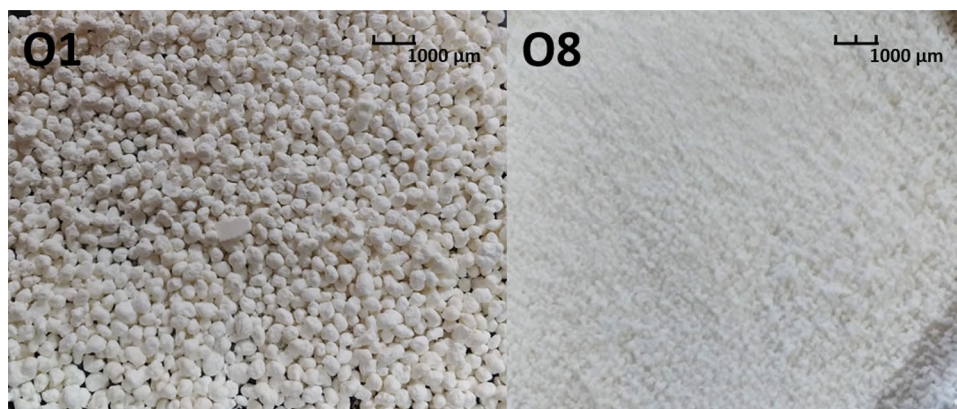
Fig. 14 Optical micrographs of PBS particles produced in soybean oil at different conditions
