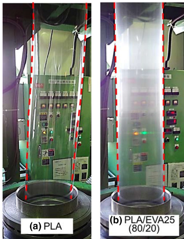
Fig. 9 Processability of tubular-blown films with 30 μm thickness
