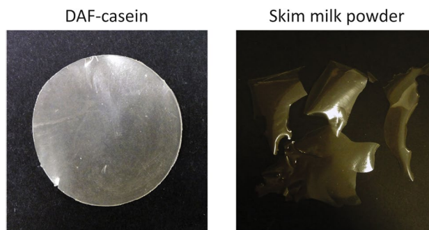
Fig. 4 Comparison of bioplastic films produced from DAF-casein and skim milk powder. DAF-casein bioplastic film produced from 2% (w/v) solution compared to a bioplastic film produced from skim milk powder
