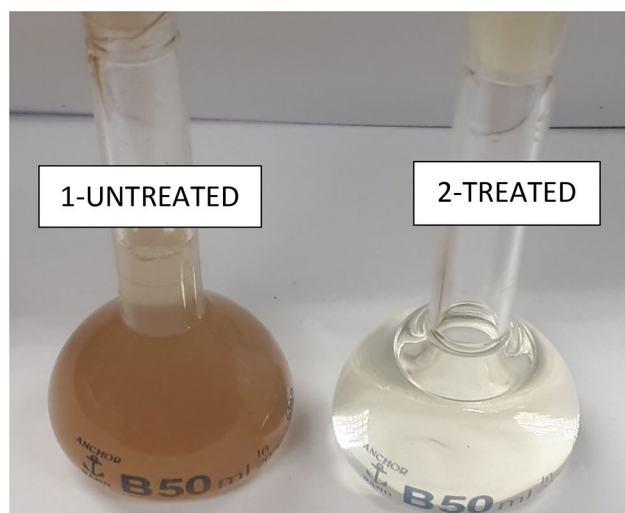
Fig. 10 Shrimp chitosan cross-linked 1,3-dichloroacetone purified poultry wastewater sample showing before treatment (1-untreated) and after treatment (2-treated)
