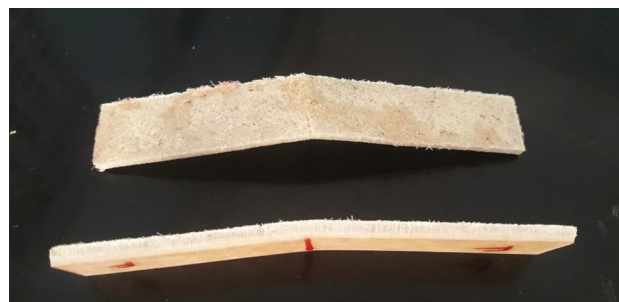
Fig. 5 Tested flexural specimen
