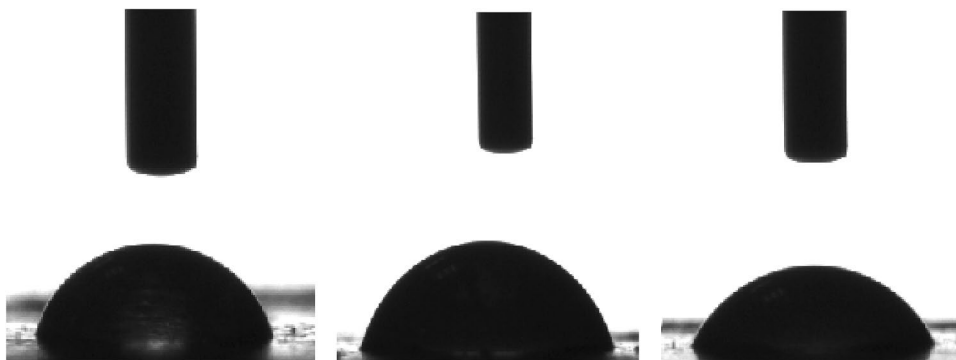
Fig. 5 The contact angle testing
