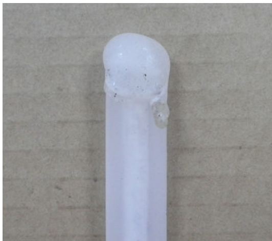
Fig. 7 Specimen combustion morphology of PP after oxygen index testing
