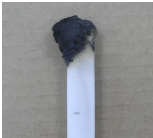
Fig. 8 Specimen combustion morphology of PP/IFR/POE/nano-CaCO 3 composite after oxygen index testing ( \phi_{IFR} = 30 wt%)
