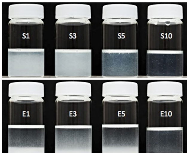
Fig. 4 TEMPO-oxidized dispersions of nanofibers from softwood and hardwood pulps with various carboxylate contents
