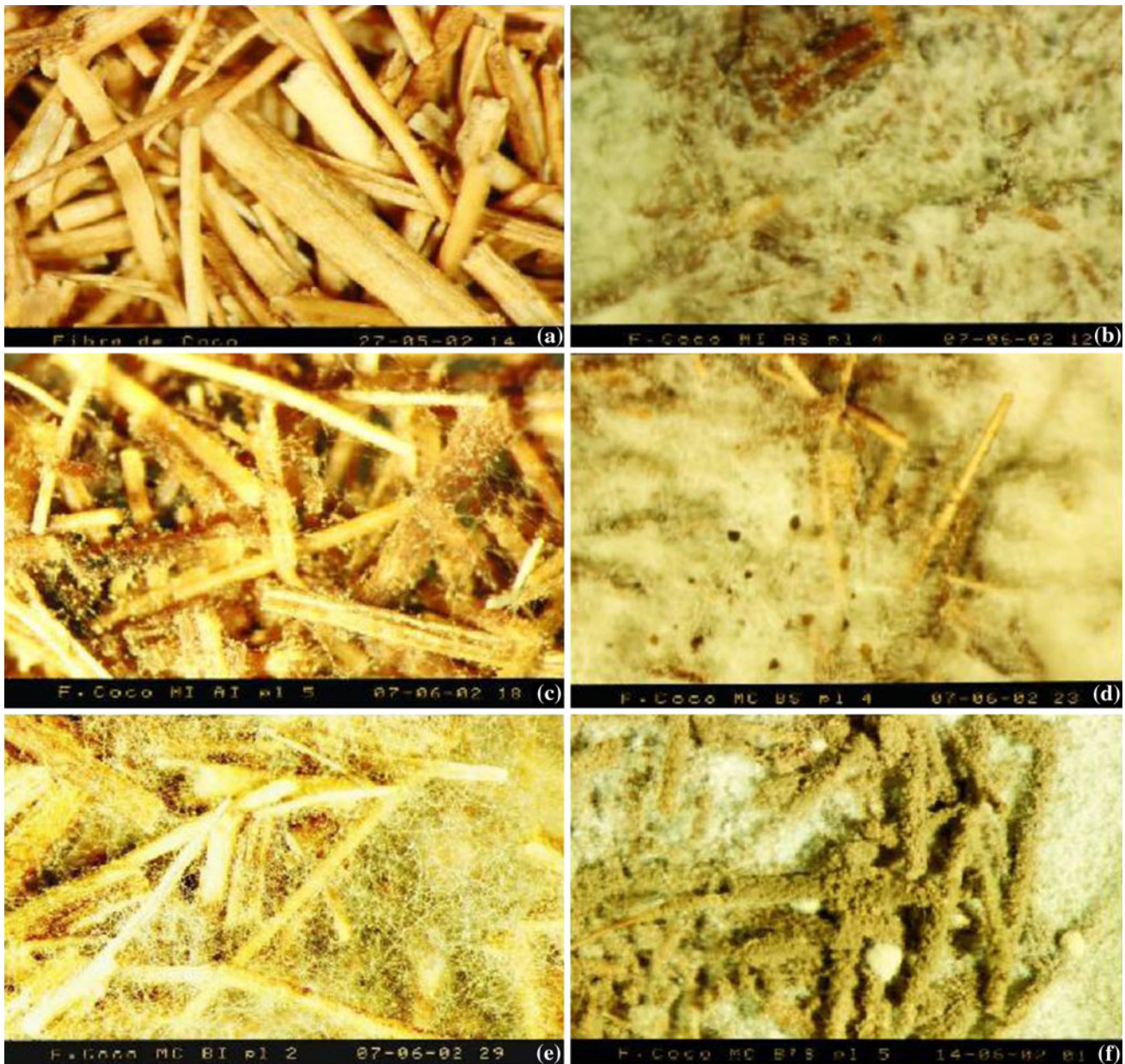
Fig. 6 Photomicrographs illustrating the coconut fiber, without inoculum and after 28 days of fungal growth ( \times 21 magnification): a without inoculum, b IM AS method, c IM AI method, d CM BS method, e CM BI method, and f CM B'S method
