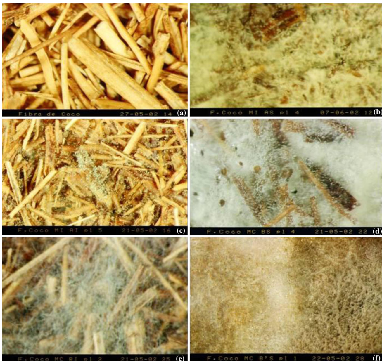
Fig. 3 Photomicrographs illustrating the coconut fiber without inoculum and after 14 days of fungal growth ( \times 13 magnification): a without inoculum, b IM AS method, c IM AI method, d CM BS method, e CM BI method, and f CM B'S method
