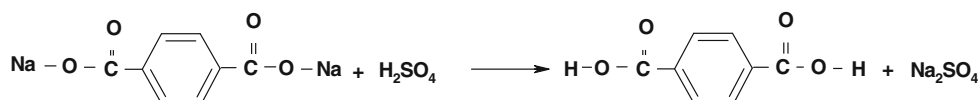
Pure TPA can be obtained by neutralisation of PET alkaline hydrolysis reaction mixture with concentrated sulfuric acid.
