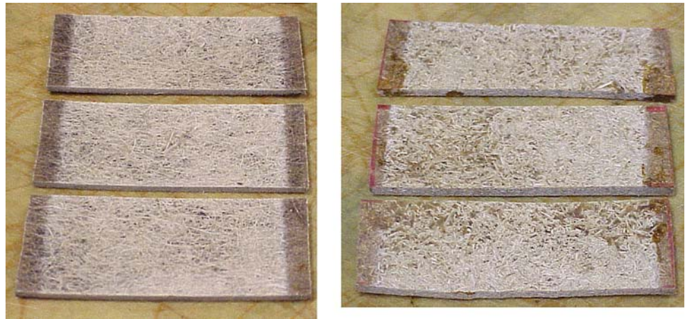
Fig. 1 Weathered samples, on left, a hemp mat-unsaturated polyester resin (UPE) biocomposite, on right, a big blue stem grass (BBSG)-GFC-UPE biocomposites
