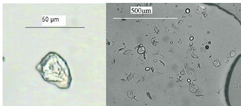
Fig. 3. PE fragments (material C) recovered from soil after centrifugation in glycerol/water solution. The observation is made by optical polarised microscopy.
