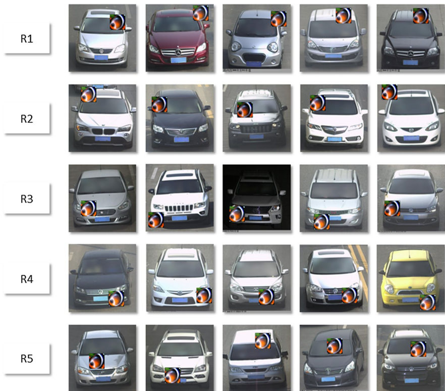
Fig. 11 (Color online) Sample vehicle images attacked with adversarial patches placed randomly within regions R1-R5 respectively (images from CompCars dataset [34])
