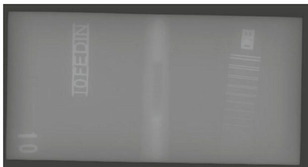
Fig. 2 The radiography image of the objects of (Fig. 1a) with root Concavity
