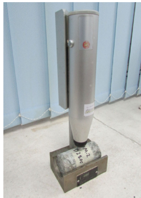
Fig. 4 A conducted test of Schmidt hammer on a sample collected from face of TBM 2
