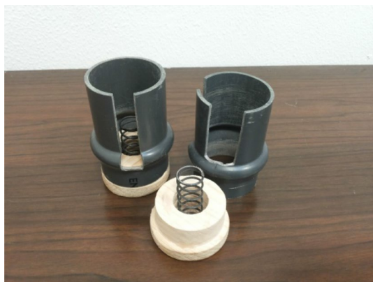
Fig. 1 Experimental tool aimed at leveling the pressure on the transducers
