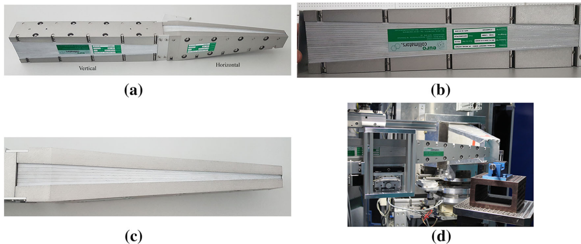
Fig. 4 a The constructed and assembled radial collimators, b side, c top view of the collimator defining the vertical and horizontal dimensions respectively, and d STRESS-SPEC setup for a test measurement where the adjustable mounting system of the primary optics (double radial collimator) is visible
