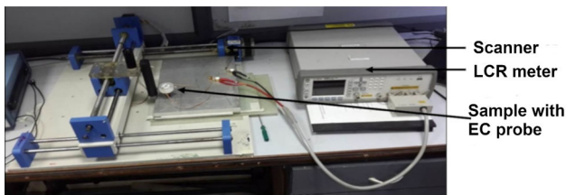
Fig. 8 ECT experimental set up
