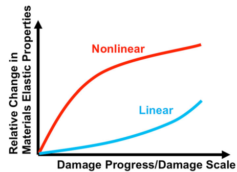
Fig. 1 Schematic evolution of nonlinear and linear elastic parameters with the damage progress or scale. Nonlinear parameters are more sensitive to early and/or microscopic damage whereas linear parameters change significantly at later stages of damage progress and are particularly useful for identifying macroscopic defects
