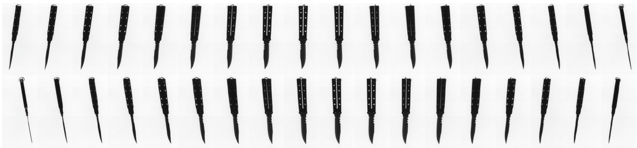
Fig. 8 A knife was rotated in 1^0 and by each position an X-ray image was captured. In this figure, X-ray images at 0^0, 10^0, 20^0, \dots, 350^0 are illustrated (see series B00008 of group Baggage)
